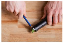
STEP 4: UNTHREAD CARTRIDGE FROM UPPER TUBE
