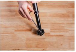
TIP: Leave front *clamp bolt* (5) & don't adjust it. When you reinstall the seat, torque the rear *clamp bolt* to 8Nm (70 in-lbs) and your seat angle will remain correct.
