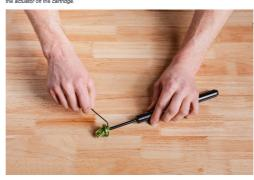
Now that the *cartridge* (15) is free from the *upper* & *lower tubes* (1,13), unthread and remove both *lock boits* (16) from the side of the *actuator* using your 2mm Hex key. Once the *lock boits* are removed you can slide the *actuator* off the *cartridge*.
