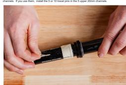
STEP 14: INSTALL PINS Remembering the orientation from when you removed them, install the guide pins (6,7) into the 6 lower 20mm channels. If you use them, install the 5 or 10 travel pins in the 5 upper 20mm channels.
