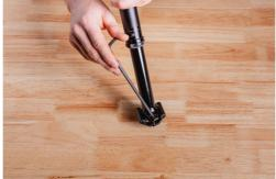
TIP: Leave front *clamp bolt* (5) & don't adjust it. When you reinstall the seat, torque the rear *clamp bolt* to 8Nm (70 in-lbs) and your seat angle will remain correct.
