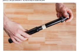
STEP 7: REMOVE LOWER TUBE Slide the lower tube (13) downward off the upper tube (1). Please note the bushings (10,11), and 6 guide pins (6,7) as you remove it, try not to drop or loose the pins.
