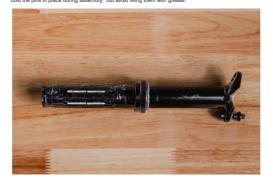
STEP 12: GREASE UPPER TUBE Using a light suspension grease (slickoleum, slick honey, SRAM butter), grease the upper tube (1) around the guide pin channels & where the lower bushing (11) will sit. Some grease in the channels is okay and can help hold the pins in place during assembly, but avoid lifting them with grease.
