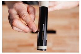
Using your pick tool, remove all the guide pins (6.7) from your upper tube (1). Wipe the grease and grit off of each pin.
