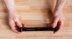
TIP: Removing the energizer from the *dust wiper* and sliding it up onto the *upper tube* before fitting the *midcap* assembly can make it easier to fit the *rubber dust wiper* onto the bottom of the *upper tube*.
