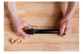
STEP 10: CLEAN AND ASSESS INTERNALS Use loopropyl alcohol and a clean cloth to wipe the upper tube (1), lower tube (13) clean. Now is a great time to assess the tubes, bushings and pins. Check for any damage, excess wear. Note: It is always recommended to rebuild your dropper with a new rebuild kit.
