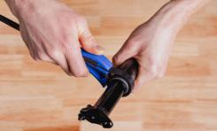
STEP 6: UNTHREAD MIDCAP ASSEMBLY Gripping the serrated collar by hand, strap wrench, or soft jaw pliers, unthread the midcap assembly (8.9) counter-clockwise. Slide the mid cap assembly up the upper tube (1)
