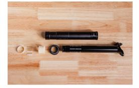
STEP 17: INSTALL ACTUATOR ON TO CARTRIDGE First ensure the *push* rod is still in your cartridge (15) and oriented with the rounded tip as the exposed end which will contact the actuator (7).
