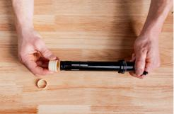
With all the guide pins (6,7) and both bushings (10,11) removed you can slide the midcap assembly (8,9) downward off the upper tube (1).
