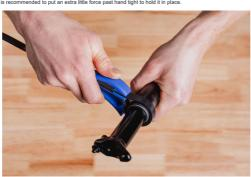
STEP 16: MID CAP ASSEMBLY With the upper bushing (10) set in place, by hand, push the midcap assembly (8,9) down onto the lower tube (13) and thread it until snug. You can thread it to hand tight if a strap wrench is not available, but it is recommended to put an extra tilt force past hand tight to hold it in place.
